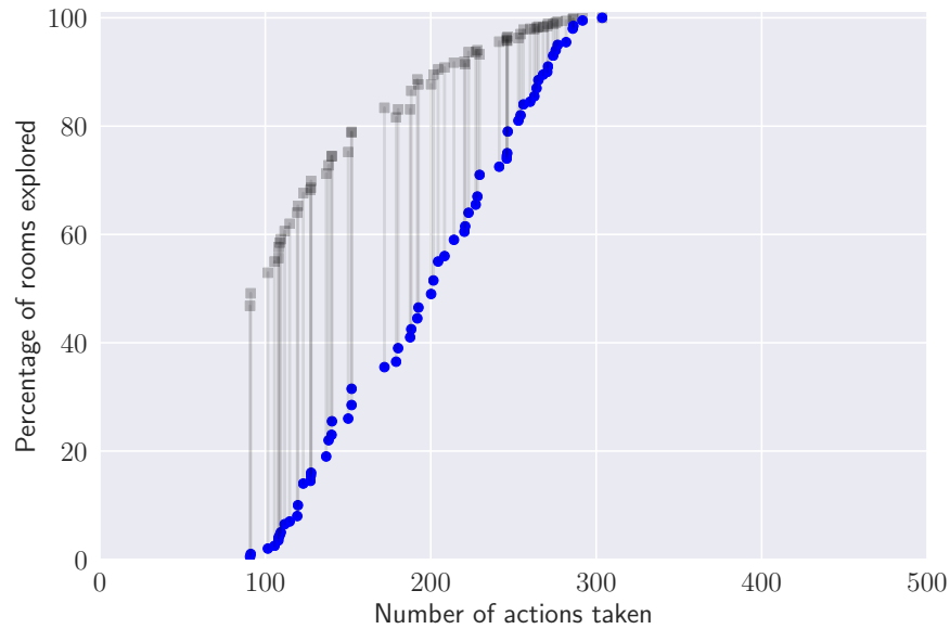
Figure 3.6 Occupancy map models with parameters that best minimize average actions per game and maximize percentage of rooms explored. Each blue dot represents the average over 200 runs using a different combination of model parameters. The blue dots show the result under the ‘exhaustive exploration’ metric and the corresponding black squares show the total percentage of rooms explored.
